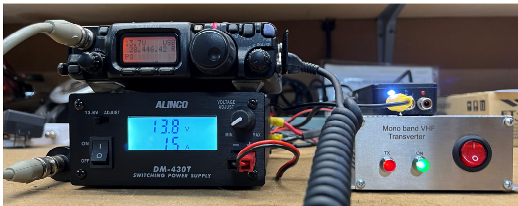
The finished PTT decoder with my FT817 and a "Ukrainian" 222 transverter
