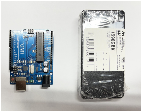
Arduino Uno is too big for the enclosure
