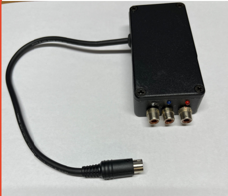
The finished PTT Decoder
